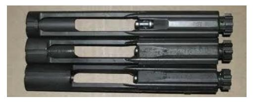
Bolt carriers came in several different styles. The most common these days is called a Full Auto Bolt Carrier which means that it has more metal at the end to theoretically trip an auto-sear once the bolt has returned to battery. The bottom one in the image is a full auto bolt carrier. In spite of the fact that these are referred to as "Full Auto" they will not convert your rifle to fully automatic and are perfectly legal in a semi-auto rifle.
