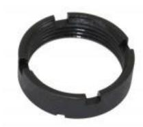
The castle nut is threaded onto the buffer tube before it is screwed into the lower receiver. Then the receiver plate is installed. Once the buffer tube has been positioned the castle nut is backed against the receiver plate and tightened with an armorer's wrench. The smaller cuts should point towards the receiver so that they can be staked into place to prevent loosening. The castle nut pictured is what typically ships with your buffer assembly kit.
