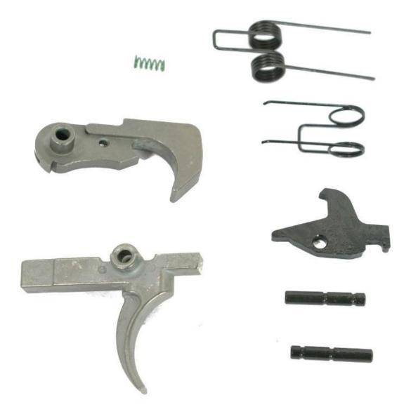
The Fire Control Group (FCG) consists of the trigger and spring, the hammer and spring the disconnect and spring and two pivot pins. The typical Milspec FCG is called a single stage trigger and can be pretty gritty and is what ships in standard LPKs. Geissele, CMC, Timney and others sell enhanced triggers with the prices starting at about \$150 and going all the way to about \$400. A \$230 2-stage trigger can greatly enhance your accuracy (prevents human error) if you want to spend the money.
