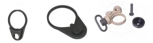
Endplates keep the buffer tube indexed (so they don't twist) and hold in the rear takedown pin detent spring, they are held in by the castle nut. They can also be purchased with different mount points. QD mount points pictured above on photo 1 and 3. The plate pictured in the middle is what typically ships with your buffer assembly kit.
