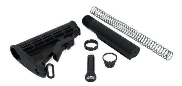
A milspec buffer tube assembly can be purchased in a kit with a standard milspec stock as pictured above. It comes with a 6-position buffer tube, buffer, buffer spring, end plate, and castle nut and the stock slides over the back of the buffer tube the buffer and spring live inside the buffer tube--the spring goes in first and is held captive by the buffer detent.
